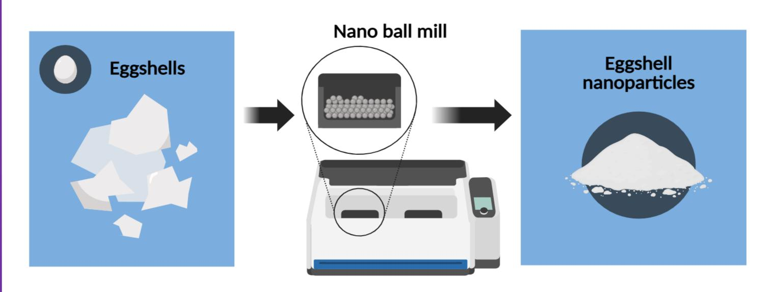
Eggshells (0.5g) were placed in a Nano mill (Retsch Co., Newton, PA) in a 50 mL stainless steel container with 50 (5 mm dia.) stainless steel balls. The eggshells were milled for 30 minutes at 15 Hz, and the powder was collected upon completion.
