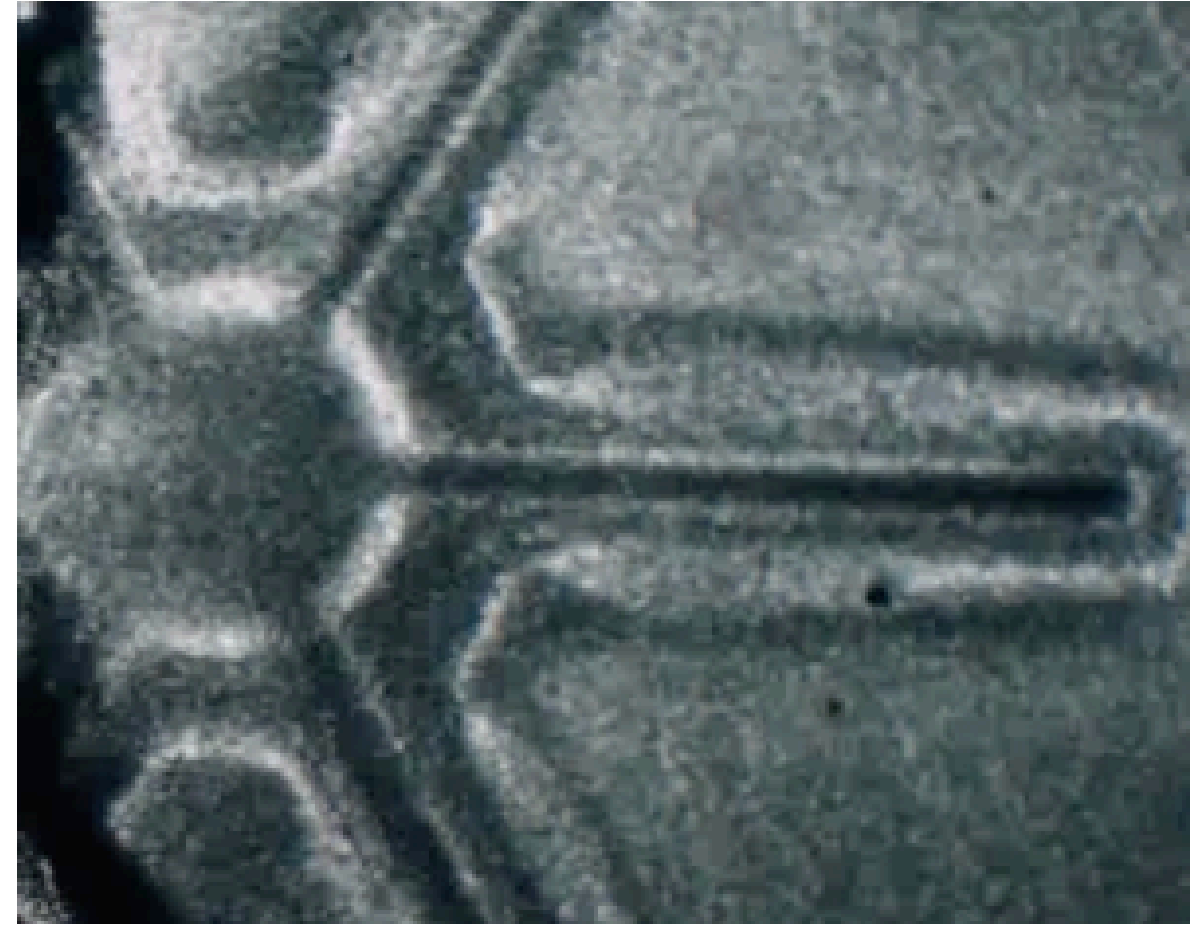
Figure 5: Higher concentration when 40 V and 9 kHz applied
