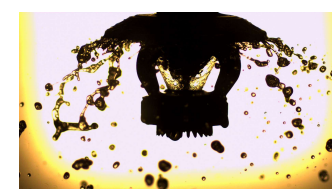
0.05% X gum + water+ biochar, GPM was steady, but feels very close to water
