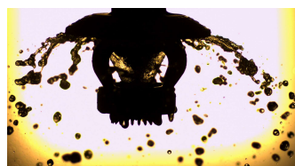
0.5% Biochar + Water, 6psi, Nozzle #8, Actual GPM=1.01GPM
