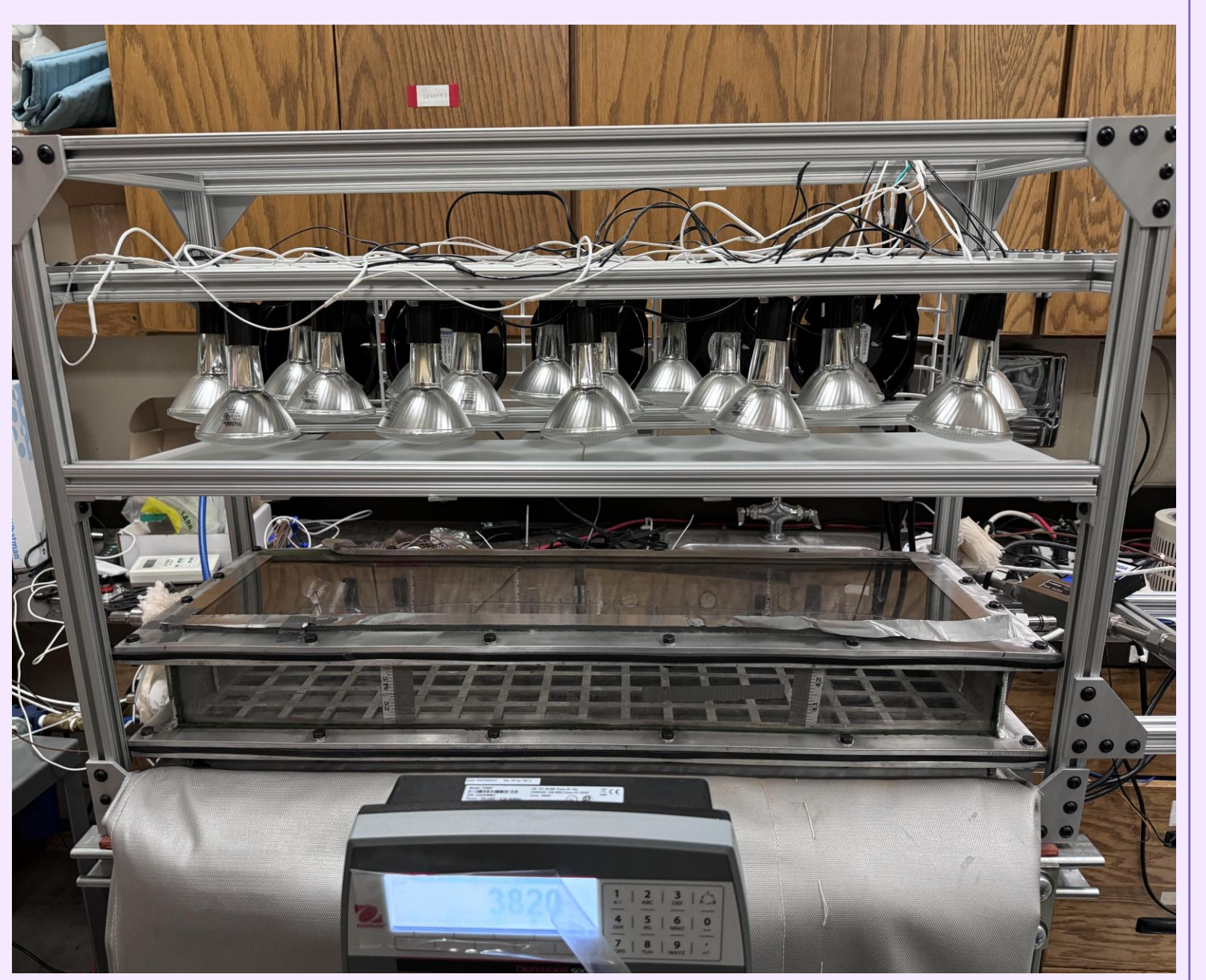
Fig 2. Experimental apparatus with simulated solar flux
