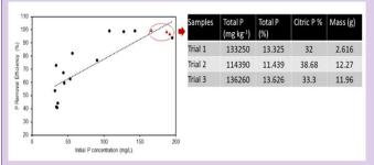
**Above Graph** demonstrates a correlation between initial P concentration (mg/L) and P Removal Efficiency (%), indicating that higher starting concentrations lead to better recovery performance.
