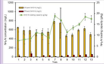
**Above Graph:** Schematic of Ammonia capture efficiency and loading capacity for clinoptilolite
